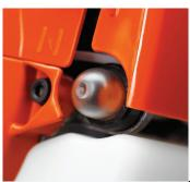
**Quick Start with Air Purge**Air purge removes air from carburetor and fuel system for easy starting
