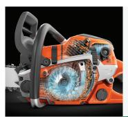
Air Injection™ Centrifugal air cleaning system for reduced wear and longer operating time between filter cleanings.
