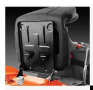
Adjustable driver seat Tool-less adjustment of seat position.
